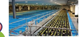
Our GeoSort is the excellent high speed machine for grading sensitive and round fruits. Large pack houses in for example Italy, Poland, United States, China, Australia and New Zealand totally rely on this grader.
