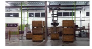
The iDA-XR HS is a high speed rotation dumper for apples and pears. The capacity is 60 bins per hour. The iDA-XR HS Q can also nest your bins; this saves you a lot of space.
